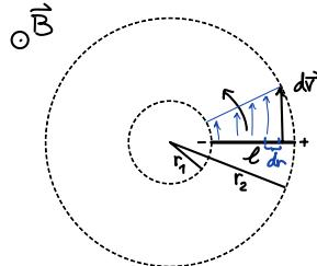
$$\begin{aligned} U_i &= \vec{v} \cdot (\vec{l} \times \vec{B}) \\ U_i &= \int dU_i = \int \vec{v} \cdot (d\vec{r} \times \vec{B}) = \int_{r_1}^{r_2} v B dr = B w \int_{r_1}^{r_2} r dr = \\ &= \frac{1}{2} B w (r_2^2 - r_1^2) = \dots = 1.57 \text{ V} \quad (T = \frac{VA}{m^2}) \end{aligned}$$
