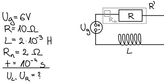
$$\underline{U_L} = L \frac{dI}{dt} = L \frac{U_g}{R'} \cdot \frac{R}{L} \exp\left\{-\frac{tR'}{L}\right\} = \\ = U_g \exp\left\{-\frac{tR'}{L}\right\} = \dots = \underline{3.3 \text{ V}}$$
