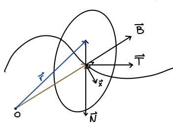
$$\underline{\vec{r}(s, r, \varphi)} = \vec{r}_K(s) + \vec{x} = \vec{r}_K(s) + r \cos \varphi \vec{N}(s) + r \sin \varphi \vec{B}(s)$$
