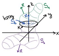
$$\partial S = K : \rightarrow \iint_S \vec{F} d\vec{S} = \iint_{S_1} \vec{F} d\vec{S} + \iint_{S_2} \vec{F} d\vec{S}$$
