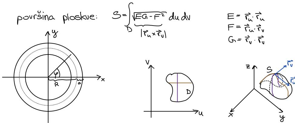
$$\text{torusne koordinate: } \begin{aligned} x &= (R + r \cos \varphi) \cos \psi \\ y &= (R + r \cos \varphi) \sin \psi \\ z &= r \sin \varphi \end{aligned}$$
