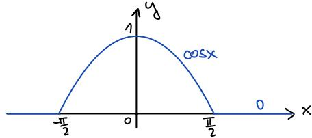
$$\underline{a_0} = \frac{1}{2\pi} \int_{-\pi}^{\pi} f(x) dx = \frac{1}{2\pi} \left[ \int_{-\pi}^{\pi/2} 0 dx + \int_{\pi/2}^{\pi} \cos x dx + \int_{\pi}^{\pi} 0 dx \right] =$$
